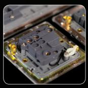
Edge to Edge Gasket Concealed edge to edge gasket to prevent tarnishing of the plate where moisture is present during installation, such as on freshly plastered or painted walls.
