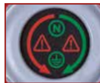
Read out dial on the reverse of plug.
