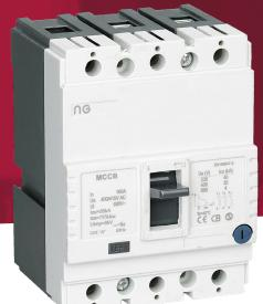
160A 4 pole MCCB combined with ELCB with adjustable thermal protection and fixed magnetic protection
