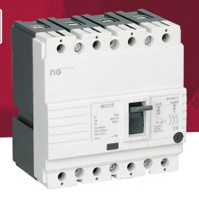
160A 4 pole MCCB with adjustable thermal protection and fixed magnetic protection
