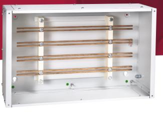
Fully rated and certified busbar chamber in steel enclosure with top and bottom blank gland plates and removable side panels. Panels fixed with key hole slots. Intended for use with the Niglon range of switch isolators and switchfuses
