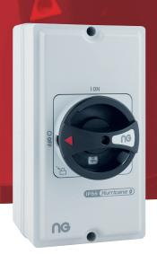
32A 4 pole switch disconnector for use with DC voltage, rated at 1500V. TUV certification. Durable polycarbonate casing with M12 knockouts, suitable for MC4 connectors. Padlockable in the off position.
