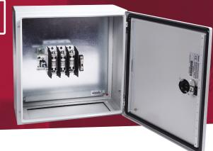
160A 3 pole switch fuse in a metal enclosure to IP65. Enclosure has separate lock and reversible door for gland plate either top or bottom. The switch handle is padlockable and defeatable. The switch fuse accepts BS88 fuse links. All terminals are provided with shrouds. Earth studs are fitted and fixing brackets and earth straps are included
