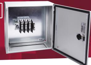
200A 3 pole switch fuse in a metal enclosure to IP65. Enclosure has separate lock and reversible door for gland plate either top or bottom. The switch handle is padlockable and defeatable. The switch fuse accepts BS88 fuse links. All terminals are provided with shrouds. Earth studs are fitted and fixing brackets and earth straps are included
