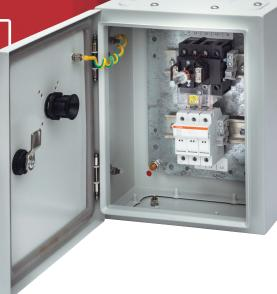
20A 3 pole fused switch in a mild steel enclosure with gland plates top and bottom. Switch handle is defeatable with provision for three padlocks. Fuse carrier accepts 10x38mm cylindrical fuselinks. Finished in epoxy powder paint, RAL 7035 colour.
