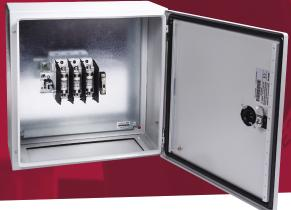
250A 3 pole switch fuse in a metal enclosure to IP65. Enclosure has separate lock and reversible door for gland plate either top or bottom. The switch handle is padlockable and defeatable. The switch fuse accepts BS88 fuse links. All terminals are provided with shrouds. Earth studs are fitted and fixing brackets and earth straps are included
