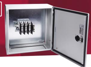
32A 3 pole switch fuse in a metal enclosure to IP65. Enclosure has separate lock and reversible door for gland plate either top or bottom. The switch handle is padlockable and defeatable. The switch fuse accepts BS88 fuse links. Terminals are integrated and shrouded. Earth studs are fitted and fixing brackets and earth straps are included
