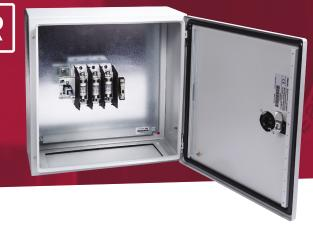
630A 3 pole switch fuse in a metal enclosure to IP66. Enclosure has separate lock and reversible door for gland plate either top or bottom. The switch handle is padlockable and defeatable. The switch fuse accepts BS88 fuse links. All terminals are provided with shrouds. Earth studs are fitted and fixing brackets and earth straps are included
