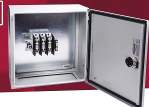
63A 3 pole switch fuse in a metal enclosure to IP65. Enclosure has separate lock and reversible door for gland plate either top or bottom. The switch handle is padlockable and defeatable. The switch fuse accepts BS88 fuse links. Terminals are integrated and shrouded. Earth studs are fitted and fixing brackets and earth straps are included
