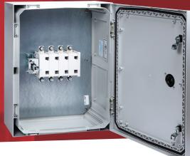
160A 4 pole switch disconnector in a glass reinforced polycarbonate enclosure to IP65 IK10. Enclosure has separate lock and reversible door. The switch handle is padlockable and defeatable. All terminals are provided with shrouds.
