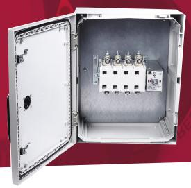
160A 4 pole manual changeover switch in a glass reinforced polycarbonate enclosure to IP65 IK10. Enclosure has separate lock. The switch handle is padlockable and defeatable.
