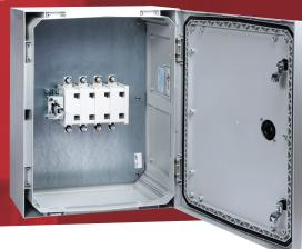
200A 4 pole switch disconnector in a glass reinforced polycarbonate enclosure to IP65 IK10. Enclosure has separate lock and reversible door. The switch handle is padlockable and defeatable. All terminals are provided with shrouds.
