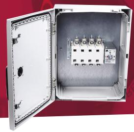
200A 4 pole manual changeover switch in a glass reinforced polycarbonate enclosure to IP65 IK10. Enclosure has separate lock. The switch handle is padlockable and defeatable.
