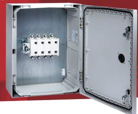
315A 4 pole switch disconnector in a glass reinforced polycarbonate enclosure to IP65 IK10. Enclosure has separate lock and reversible door. The switch handle is padlockable and defeatable. All terminals are provided with shrouds.
