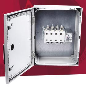
315A 4 pole manual changeover switch in a glass reinforced polycarbonate enclosure to IP65 IK10. Enclosure has separate lock. The switch handle is padlockable and defeatable.
