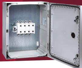
400A 4 pole switch disconnector in a glass reinforced polycarbonate enclosure to IP65 IK10. Enclosure has separate lock and reversible door. The switch handle is padlockable and defeatable. All terminals are provided with shrouds.
