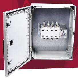
400A 4 pole manual changeover switch in a glass reinforced polycarbonate enclosure to IP65 IK10. Enclosure has separate lock. The switch handle is padlockable and defeatable.
