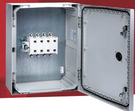
630A 4 pole switch disconnector in a glass reinforced polycarbonate enclosure to IP66 IK10. Enclosure has separate lock and reversible door. The switch handle is padlockable and defeatable. All terminals are provided with shrouds.
