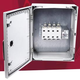
630A 4 pole manual changeover switch in a glass reinforced polycarbonate enclosure to IP65 IK10. Enclosure has separate lock. The switch handle is padlockable and defeatable.
