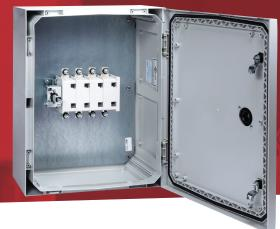
800A 4 pole switch disconnector in a glass reinforced polycarbonate enclosure to IP65 IK10. Enclosure has separate lock and reversible door. The switch handle is padlockable and defeatable. All terminals are provided with shrouds.
