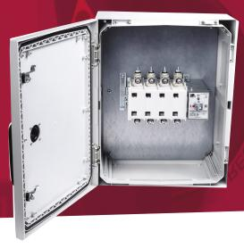
800A 4 pole manual changeover switch in a glass reinforced polycarbonate enclosure to IP65 IK10. Enclosure has separate lock. The switch handle is padlockable and defeatable.
