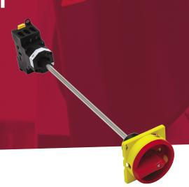
125A 3 pole door interlock switch disconnector comprising din rail mount switch, metal shaft and handle. Handle is padlockable in the off position and has provision for 3
