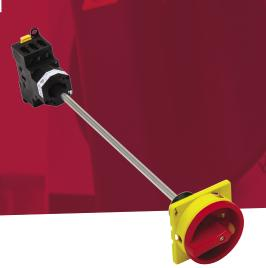
80A 3 pole door interlock switch disconnector comprising din rail mount switch, metal shaft and handle. Handle is padlockable in the off position and has provision for 3
