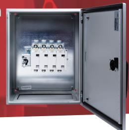
160A 4 pole switch disconnector in a stainless steel enclosure to IP65. Enclosure has separate door lock. The switch handle is padlockable and defeatable. All terminals are provided with shrouds. Earth studs are fitted and fixing brackets and earth straps are included
