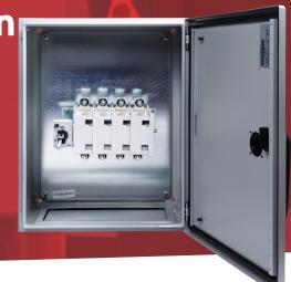
250A 4 pole switch disconnector in a glass reinforced polycarbonate enclosure to IP65 IK10. Enclosure has separate lock and reversible door. The switch handle is padlockable and defeatable. All terminals are provided with shrouds.
