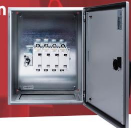
315A 4 pole switch disconnector in a metal enclosure to IP65. Enclosure has separate lock and reversible door. The switch handle is padlockable and defeatable. All terminals are provided with shrouds. Earth studs are fitted and fixing brackets and earth straps are included
