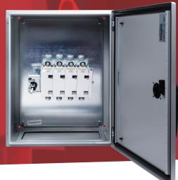
400A 4 pole switch disconnector in a metal enclosure to IP65. Enclosure has separate lock and reversible door. The switch handle is padlockable and defeatable. All terminals are provided with shrouds. Earth studs are fitted and fixing brackets and earth straps are included
