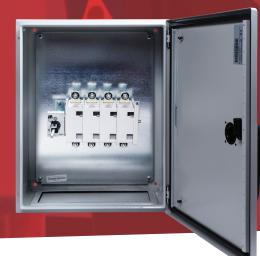
630A 4 pole switch disconnector in a metal enclosure to IP65. Enclosure has separate lock and reversible door. The switch handle is padlockable and defeatable. All terminals are provided with shrouds. Earth studs are fitted and fixing brackets and earth straps are included
