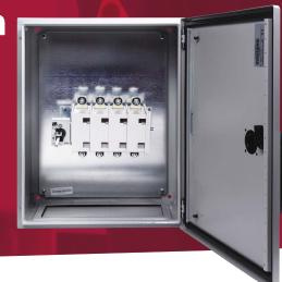
1000A 4 pole switch disconnector in a metal enclosure to IP66. Enclosure has separate lock and reversible door. The switch handle is padlockable and defeatable. All terminals are provided with shrouds. Earth studs are fitted and fixing brackets and earth straps are included
