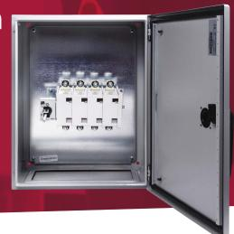
1250A 4 pole switch disconnector in a metal enclosure to IP66. Enclosure has separate lock and reversible door. The switch handle is padlockable and defeatable. All terminals are provided with shrouds. Earth studs are fitted and fixing brackets and earth straps are included
