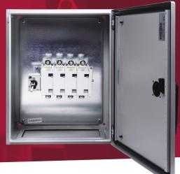
800A 4 pole switch disconnector in a metal enclosure to IP66. Enclosure has separate lock and reversible door. The switch handle is padlockable and defeatable. All terminals are provided with shrouds. Earth studs are fitted and fixing brackets and earth straps are included
