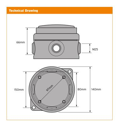
General purpose junction box suitable for all surface industrial applications. It is manufactured from impact, corrosion and UV resistant glass reinforced polyester compound.
