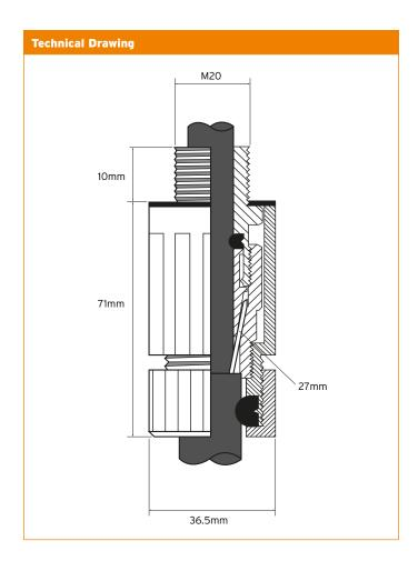
For use in highly corrosive and wet locations. The screw on shroud is manufactured from corrosion resistant non-metallic material, providing total enclosure of the steel wire armour and metal parts of the gland.
