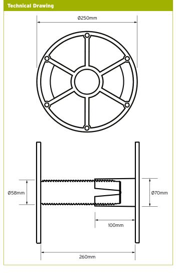
Conceived and developed out of the necessity to stop wasting time and money caused by damaged cable drums. The reelsaver is manufactured from fully recyclable ABS and polycarbonate materials.
