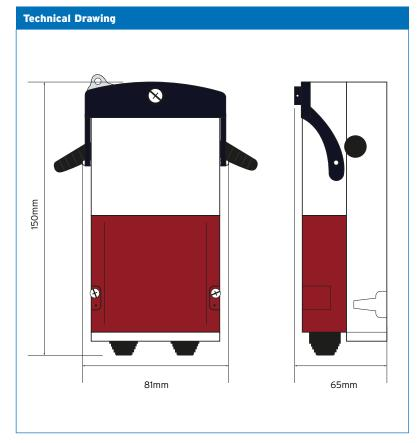
DP single phase, single fuse, with earth block and brass plate. 2 x 20mm grommets
