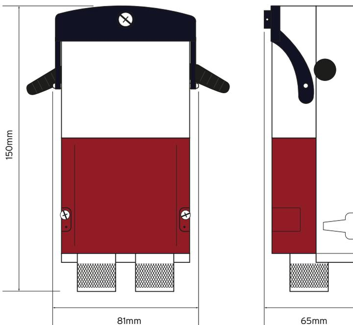
DP single phase, double pole fuse with earth block and brass plate. 2 x 20mm tubes
