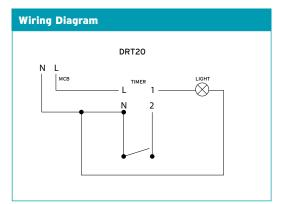
The DRT20 is a variable delay timer to control stairwell lighting.
