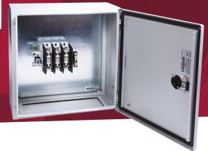
100A 3 pole switch fuse in a metal enclosure to IP65. Enclosure has separate lock and reversible door for gland plate either top or bottom. The switch handle is padlockable and defeatable. The switch fuse accepts BS88 fuse links. All terminals are provided with shrouds. Earth studs are fitted and fixing brackets and earth straps are included
