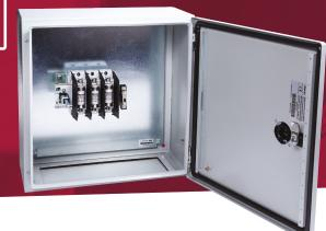
125A 3 pole switch fuse in a metal enclosure to IP65. Enclosure has separate lock and reversible door for gland plate either top or bottom. The switch handle is padlockable and defeatable. The switch fuse accepts BS88 fuse links. All terminals are provided with shrouds. Earth studs are fitted and fixing brackets and earth straps are included
