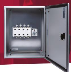
160A 4 pole manual changeover switch in a metal enclosure to IP65. Enclosure has separate lock. The switch handle is padlockable and defeatable. Earth studs are fitted and fixing brackets and earth straps are included
