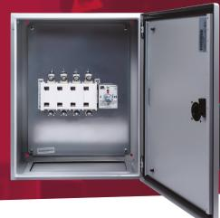
1800A 4 pole manual changeover switch in a metal enclosure to IP65. Enclosure has separate lock. The switch handle is padlockable and defeatable. Earth studs are fitted and fixing brackets and earth straps are included
