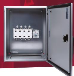
250A 4 pole manual changeover switch in a glass reinforced polycarbonate enclosure to IP65 IK10. Enclosure has separate lock. The switch handle is padlockable and defeatable.
