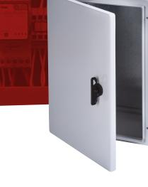
Wall mounting mild steel enclosure painted with epoxypolyester powder paint. Standard RAL7035 colour. The polyurethane gasket keeps its profile over time to give a high degree of protection against water and dust. Door opens 125° and is reversible. One gland plate can be top or bottom. Welded earth studs top and bottom. Fitted, galvanised backplate has return edges for extra rigidity.
