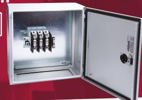
315A 3 pole switch fuse in a metal enclosure to IP65. Enclosure has separate lock and reversible door for gland plate either top or bottom. The switch handle is padlockable and defeatable. The switch fuse accepts BS88 fuse links. All terminals are provided with shrouds. Earth studs are fitted and fixing brackets and earth straps are included
