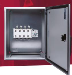
315A 4 pole manual changeover switch in a metal enclosure to IP65. Enclosure has separate lock. The switch handle is padlockable and defeatable. Earth studs are fitted and fixing brackets and earth straps are included
