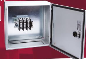
400A 3 pole switch fuse in a metal enclosure to IP65. Enclosure has separate lock and reversible door for gland plate either top or bottom. The switch handle is padlockable and defeatable. The switch fuse accepts BS88 fuse links. All terminals are provided with shrouds. Earth studs are fitted and fixing brackets and earth straps are included
